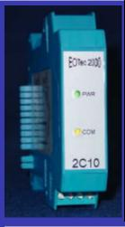
The 2C10 Module provides RS-232 or RS-485 electrical interface conditioning for data transmission over the fiber optic network. The module can be selected to support either point-to-point RS-232 or multi-drop RS-485 half-duplex communications at baud rates up to 230K.
